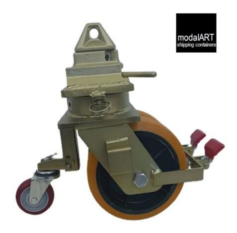
Engineered for heavy-duty applications, these casters handle dynamic loads up to **13,500 KG** and static loads up to **18,000 KG**. They attach securely to ISO container corners using a twistlock system for easy installation.
